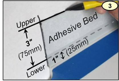
**1.** Clean the rim with alcohol wipes. **2.** Apply painters tape over the rim 9/32" (7mm) out from walls. **3.** Twice apply 2 wall marks to each wall at 3" (75mm) and 1" (25mm) above the rim.
